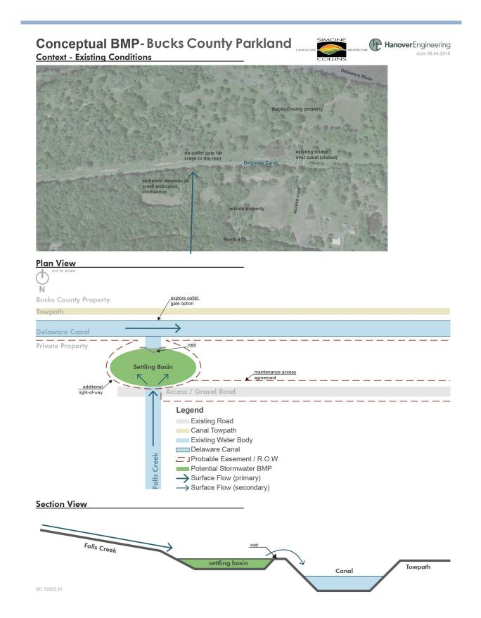
**Bucks County Parkland as a Model BMP:** The concept of catching sediments and allowing for regular maintenance / cleanout of these settling basins might be considered where watercourse confluences with the Delaware Canal exist as a strategy to preempt sediment deposits into the canal flow and enable proactive maintenance directly up-watershed from the canal.
