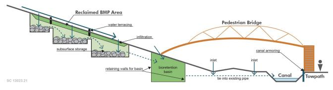
Closer to the Highlands Boulevard and PA Route 611 intersection, water might be piped from the roadside BMP to bio-retention basins, where it would be stored and released slowly. If excess stormwater fills the basins, the water outfalls into pipes that tie into the existing stormwater systems and discharge into the canal. The goal is to slow velocity and allow for longer detention than pre-design conditions.
