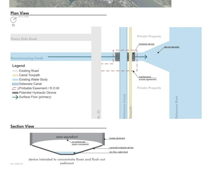
**Paunacussing Creek and Aqueduct as a Model BMP:** Paunacussing Creek has an extreme case of sediment deposits near and under a Delaware Canal aqueduct. The addition of a hydraulic device may not be appropriate in other locations.
