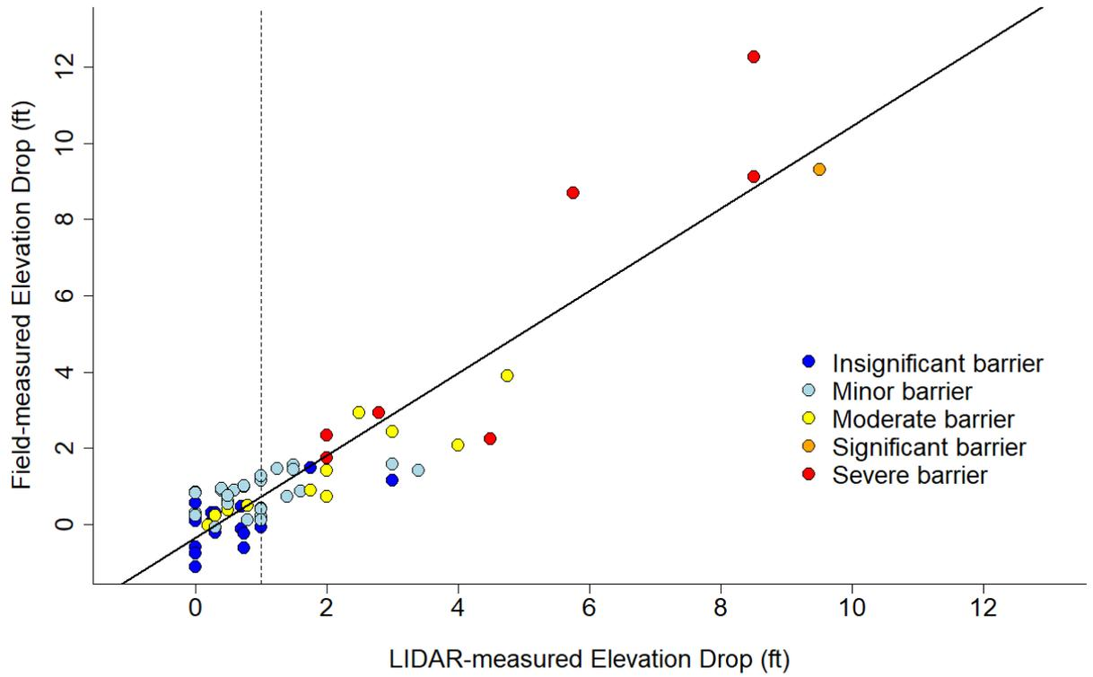
Figure 3. Computer-based assessments of fish passage at road-stream crossings identified 107 potential barriers to fish passage (black points) in 9 LDWS municipalities. 62 of these potential barriers were in wild trout waters, and TU staff's initial review identified 34 potential barriers to study further for their potential benefit to wild trout populations (red points).
