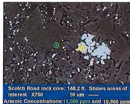
Figure 6. Electron micrograph at 750 times magnification showing pyrite (light) and calcite (dark). Green and yellow circles show pyrite grains with 11,500 ppm and 15,860 ppm arsenic respectively. Rock has 130 ppm As. (Core sample courtesy Zoltan Szabo, USGS).
