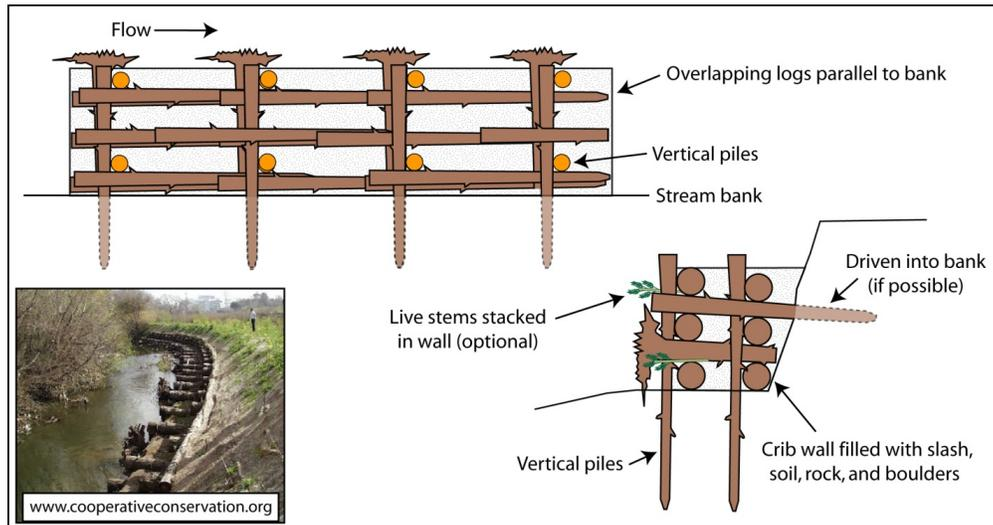
Figure 11. Examples of nature-based solutions for bank stabilization include a) brush mattresses for low energy environments and b) log crib walls for higher energy settings.
